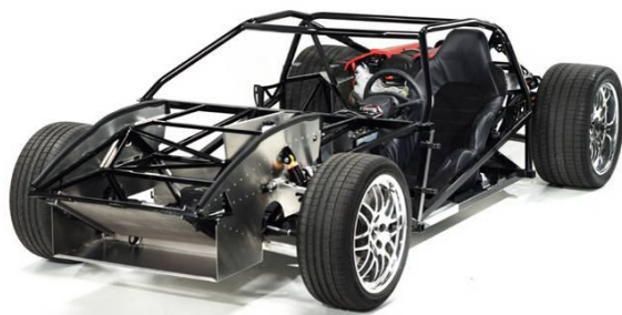
Figure 3: Example of real rolling chassis without aero parts.
